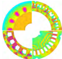
Motor design: topology and simulation-driven optimization for maximum power density
