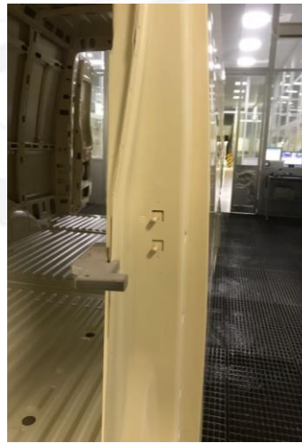
sliding door stopper in PEEK
