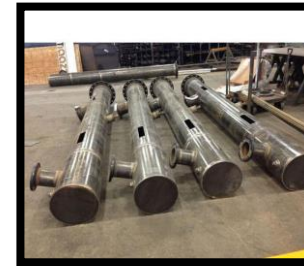
Header piping system
