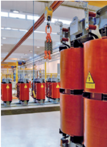
Cast resin transformers production plant
