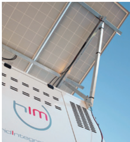
Hybrid gensets with solar energy integration
