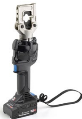
Battery-powered hydraulic crimping tool, 68kN, bi-linear, with closed openable head, for electrical connectors up to 300 mm 2
