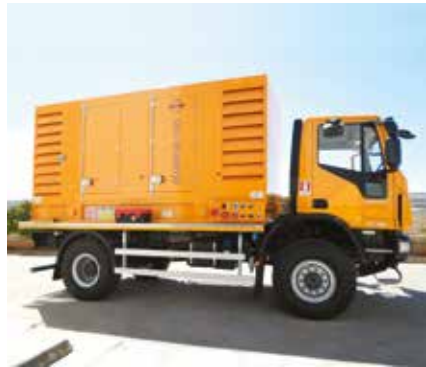
DGS on 4x4 truck for power generations in remote areas, Disaster & Recovery applications and Airports with single/dual/parallel operation
