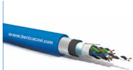
CU/MGT/XLPE/OSCR/LSZH/SWA/LSZH
