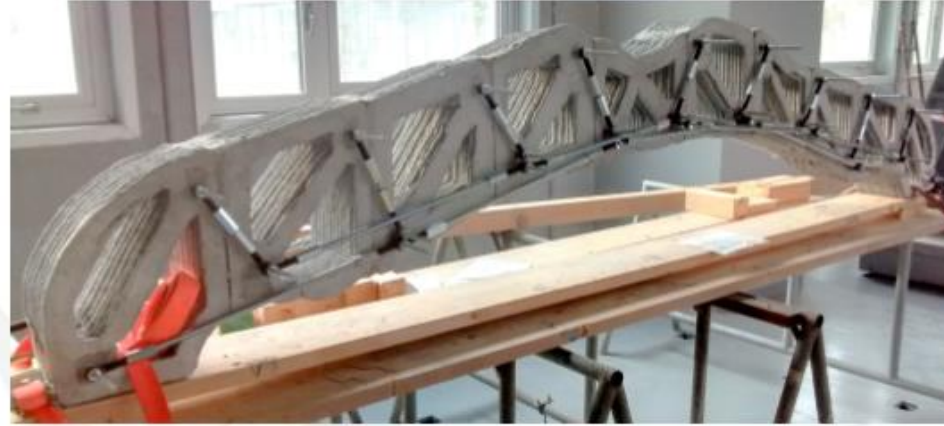
Vesuvio RC Beam: 3D printing
