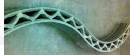
3D printed curve wall, University of Southern California
