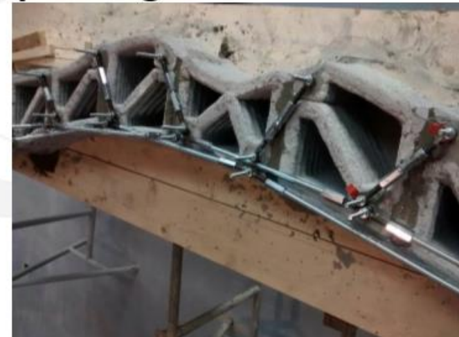
Vesuvio RC Beam: 3D printing
