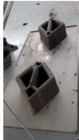
Vesuvio RC Beam: 3D printing
