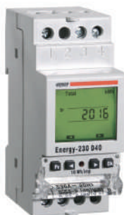
Single-phase active energy meter (bidirectional measure for both produced and consumed energy) on 2 DIN rail modules case with pulse output for remote control.
