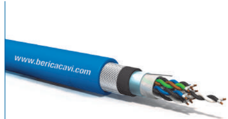
CU/MGT/XLPE/OSCR/LSZH/SWA/LSZH
