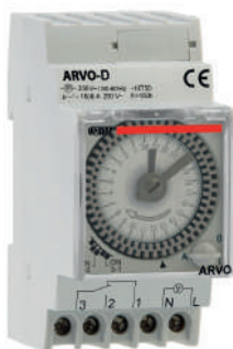
DIN-rail electromechanical daily time switch with trippers (15 min resolution) and back-up-battery (replaceable)
