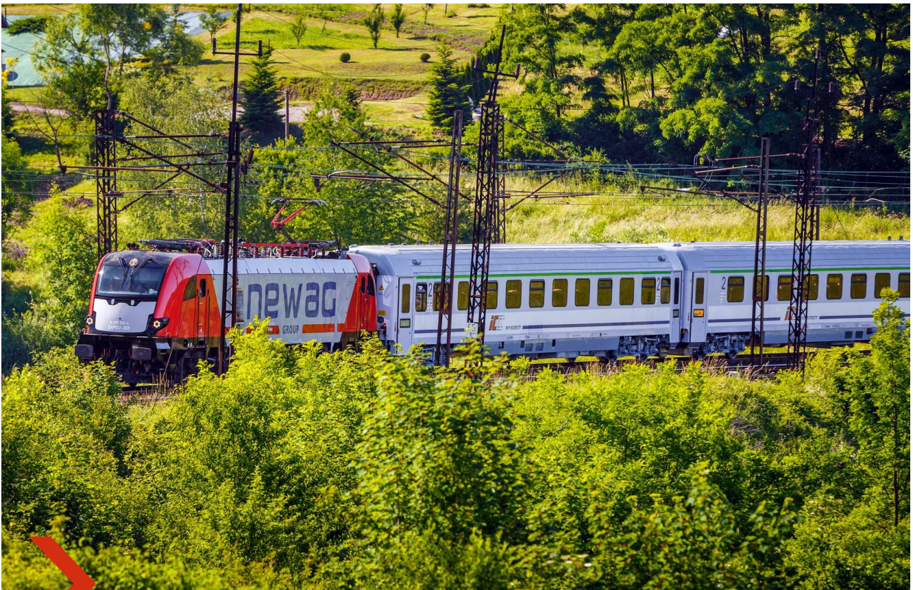
Griffin E4MSFDP - R&D Project 4-axle multisystem electric locomotive(NC BiR)
