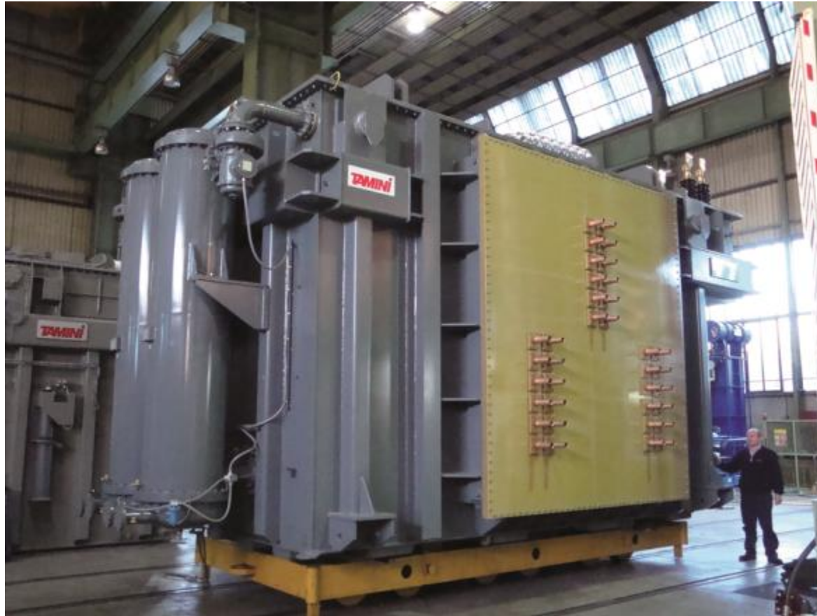
ATAKAS - EAF Transformer 360 MVA - 34500/1680-1600-1100 V The biggest EAF Transformer in the World
