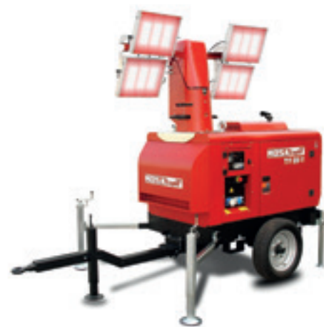
TF 119 Y L-4x250: 9m zinc plated telescopic mast, 4 x 250W LED lamps, hydraulic raise/lower, with generator integrated, engine Diesel YANMAR 3TNV76, single-phase power 6.5 kVA, LED light
