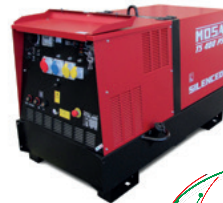
TS 400 PS BC: Diesel Engine driven welder - PERKINS 404A-22G1 Engine - Three-phase asynchronous alternator - Three-phase generation 16 kVA - Single-phase generation 12 kVA - Max welding current: 400A
